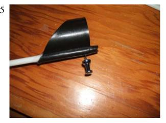
Roll the shaft a little and then push down the tape lengthwise. Do this in increments. Each time you push down on the tape, you will stick a little bit more of the tape to the shaft.
