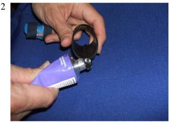
If the end of the shaft has spread due to hammering, lightly sand the edge to bring it back to the right size so the APD will fit. Do not reduce the shaft diameter with sanding.
