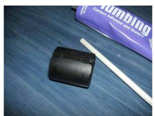
Glue the APD onto the bolt shaft by placing glue into the groove, then placing your clean bolt shaft into the glue filled groove and waiting for the glue to harden. The glue holds it in place so you easily tape it. Fast drying glue from a hot melt glue gun works great.
