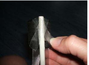
Do the same with the other 3 split ends forming X's. Pull the tape TIGHT. Repeat with another 6-inch strip of split tape over the first.
