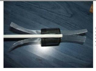
Feed this through the APD so it sticks out evenly on either end. The sticky part of the tape needs to contact the inside of the APD.
