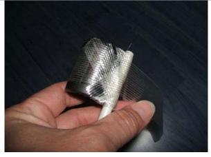
Wrap strapping tape (pull tight) twice around the whole thing, and then cover with electrical tape.
